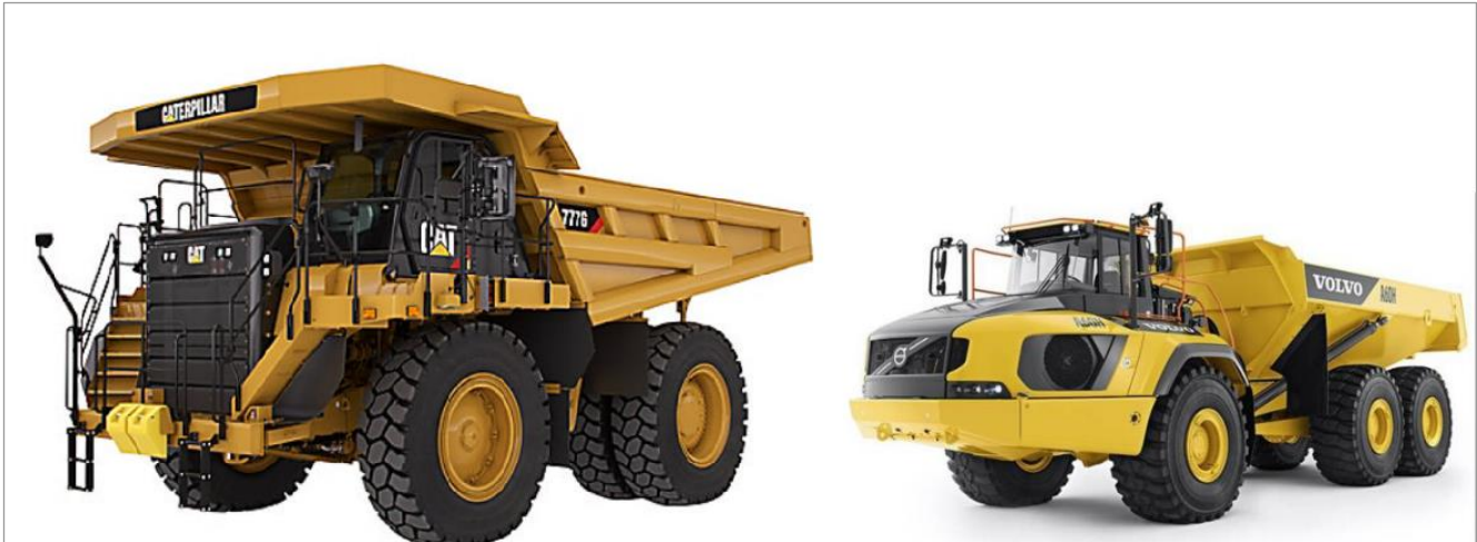
Figure 16.7 Graphic showing type of trucks selected (CAT 777 90 t and Volvo A60H 55 t trucks)
